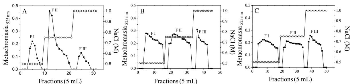
**Figure 2.** Ion-exchange chromatography (DEAE-cellulose) of TSPs from green marine algae *Caulerpa racemosa* (A), *Caulerpa prolifera* (B) and *Caulerpa cupressoides* (C). The column was balanced and eluted with 50 mM sodium acetate buffer (pH 5.0). The SPs adsorbed on the gel were eluted with the addition of NaCl (0.50, 0.75 and 1.00 M). (■—■) metachromasia; (○—○) NaCl concentration (M).
